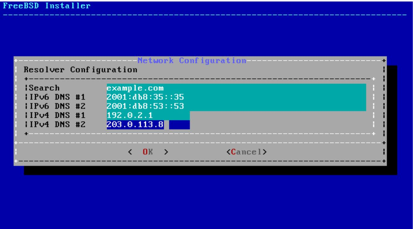
Figure 59. DNS Configuration
