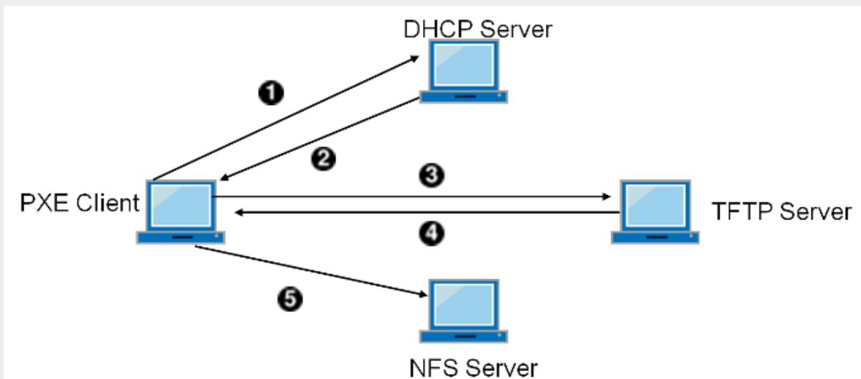
Figure 61. PXE Booting Process with NFS Root Mount
